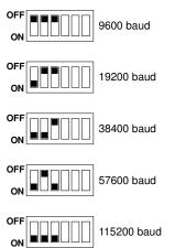
The dip switches used to select the speed and mode of the converter are situated next to the RS232 connection cable
