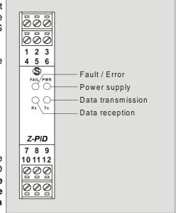
The wiring of the power supply and serial bus is facilitated by the use of a support bus that can be lodged within the DIN guide. Such a system also allows for hot swapping, that is, the insertion and extraction of the module from the bus without the interruption of the communication nor the power supply to the remaining part of the system.
