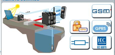
Remote control with Z-PC means having an integrated system based on a broad spectrum of RTUs (all-in-one, battery powered, small systems and cathodic protection), standard protocol and libraries of specific functions dedicated to the remote control applications.
