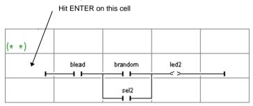
The ISaGRAF Quick LD editor keeps the memory of the rung labels you already entered, whether it has been specified for a rung name or a jump operation. The "Jump/Label" dialog box gives you the possibility either to enter a new label, or to select an existing one.
