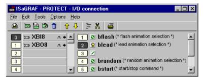
Use the "Set protection" and "Remove protection" commands of the "Edit" menu to set or remove an individual protection for selected channel. Both commands ask you to enter a valid password so that a protection level can be attached to the channel. Then, each time you want to change connection to a channel having individual protection you must enter a password with sufficient priority level.
