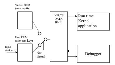
Setting the virtual attribute follows the same rules for an input board or an output board. For output boards, the ISaGRAF kernel updates the output database. This database and the associated output devices are, however, disconnected. A virtual I/O driver replaces the real one.
