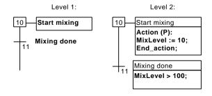
The level 2 programming of a step is entered in a text editor. It can include action blocks programmed in ST or IL. The level 2 programming of a transition can be entered either in IL or ST text languages, or with Quick LD editor.
