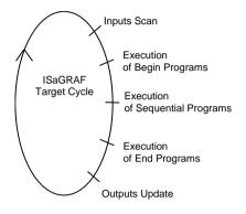
The target cycle consists in scanning the physical inputs of the process to drive, processing application data according to the ISaGRAF workbench<sup>1</sup> application programs and then performing physical outputs update.
