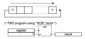
(\* ST Equivalence: \*) result := ROR (register, 1); (\* register = 2#0100\_1101\_0011\_0101 \*) (\* result = 2#1010\_0110\_1001\_1010 \*)
